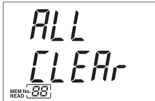
ALL CLEAR alarm indication
