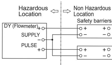
[Remote type without built-in Temperature sensor]
