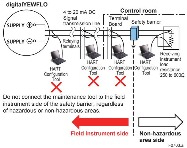
Do not connect the maintenance tool to the field instrument side of the safety barrier, regardless of hazardous or non-hazardous areas.
