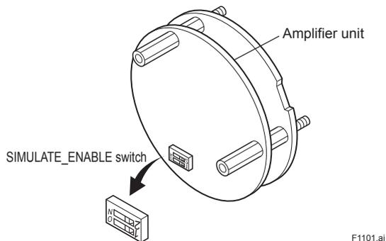
Figure 11.1 Amplifier for Fieldbus Communication
