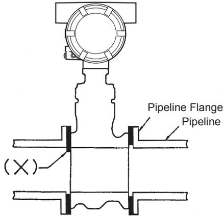
2. Avoid mounting gaskets which protrude into the pipeline. This may cause inaccurate readings. Use gaskets with bolt holes, even if digitalYEWFL0 is of the wafer type. When using a spiral gasket (without bolt holes), confirm the size with the gasket-manufacturer, as standard items may not be used for certain flange ratings.
