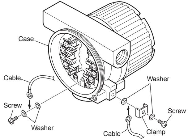
(1) Internal grounding terminal (2) External grounding terminal F1004.ai
