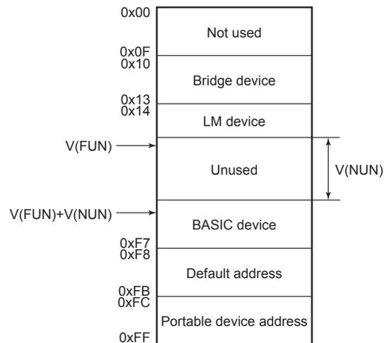
Note 1: LM device: with bus control function (Link Master function)
