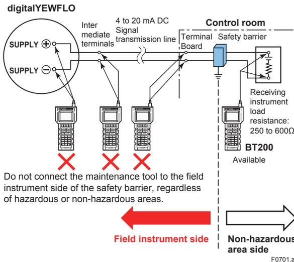
Figure 7.1 Communicating for a 4 to 20mA DC Signal Line
