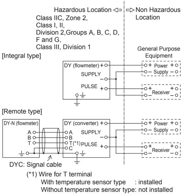
Non-incendive field wire parameters of vortex flowmeter (DY) and converter (DYA).
