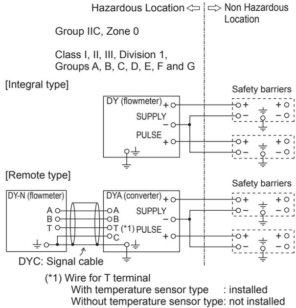
Electrical parameters of vortex flowmeter (DY) and converter (DYA).
