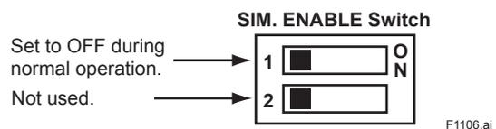
**Figure 11.6 SIMULATE\_ENABLE Switch Position**
