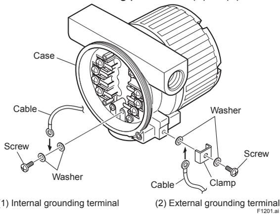
**Figure 12.1 Wiring Procedure for Grounding Terminals for Flameproof**
