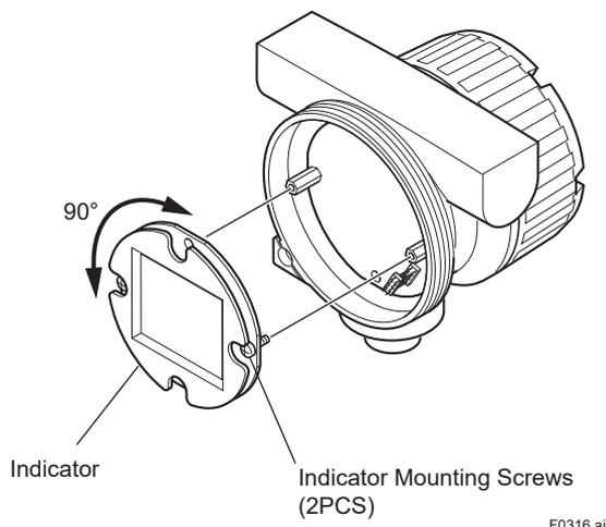
Figure 3.2 Removing and Reinstalling the Indicator
