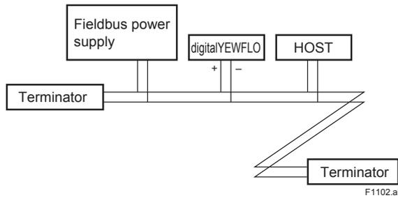
Figure 11.2 Device Connection
