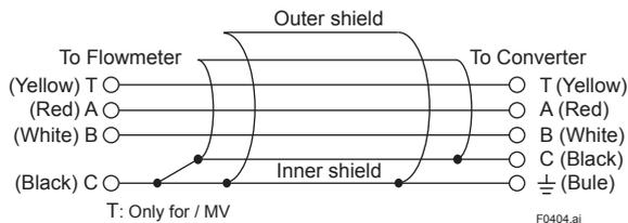
Figure 4.5 Construction of DYC Remote Type Signal Cable
