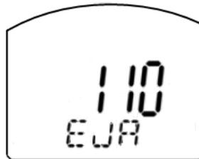
Model of Transmitter (3 seconds)
