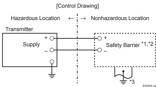
\*1: In any safety barrier used output current must be limited by a resistor 'R' such that  $I_o = U_z/R$ .
