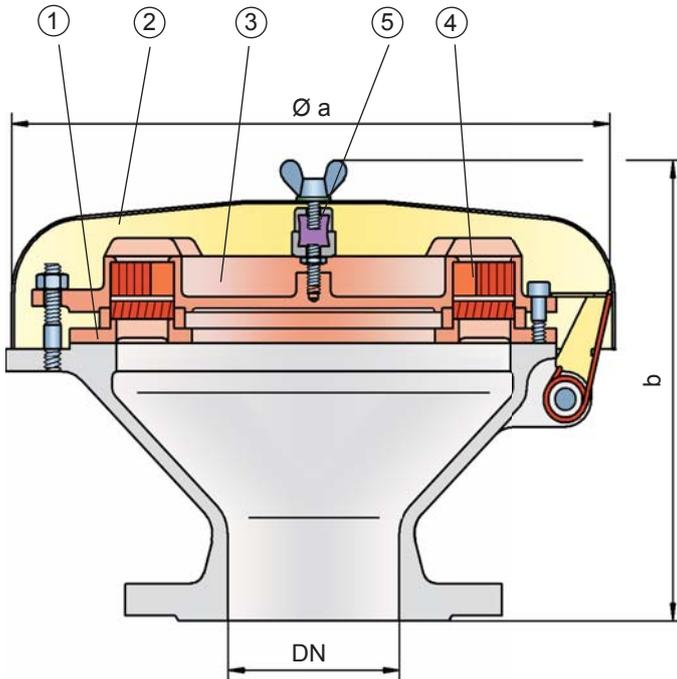
The PROTEGO® BE/HR-E end-of-line deflagration flame arrester is available for hydrocarbons for explosion group IIB (MESG  $\geq 0,5$  mm) and alcohols.
