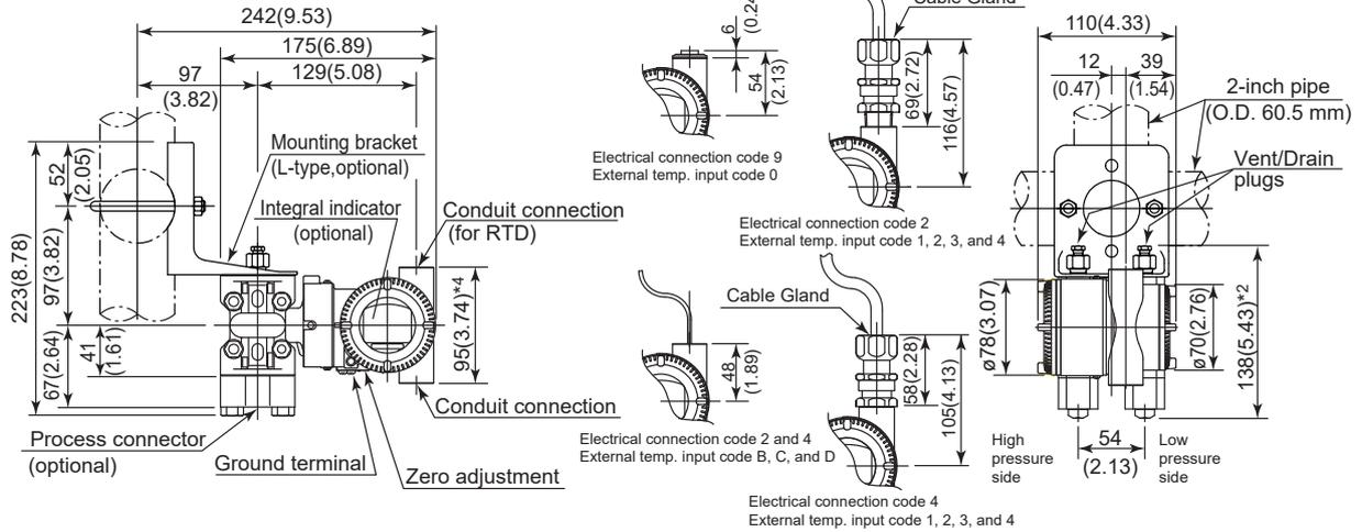
● Horizontal Impulse Piping Type (Installation code 9)
