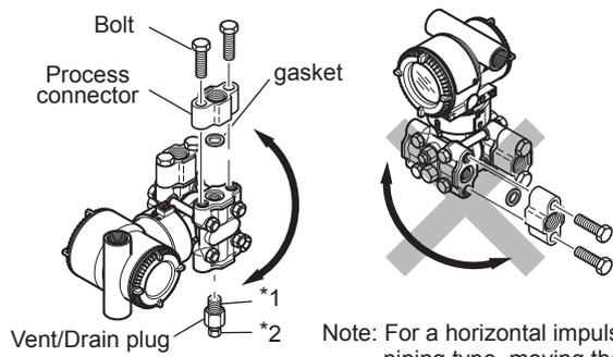
Note: For a horizontal impulse piping type, moving the process connectors from the front side to the back is not allowed.
