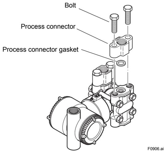
Figure 9.6 Removing and Mounting the Process Connector
