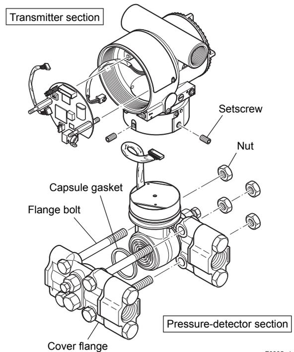
**Figure 9.5 Removing and Mounting the Pressure-detector Section**
