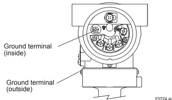
Figure 7.12 Ground Terminals (Eg. HART Communication Type)
