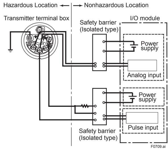
Figure 7.7 Connection between Transmitter, barrier and receiver
