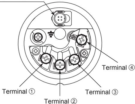
● Terminal Wiring (HART and FOUNDATION Fieldbus protocol types)
