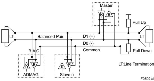
**Figure 5.2 Modbus connection**
