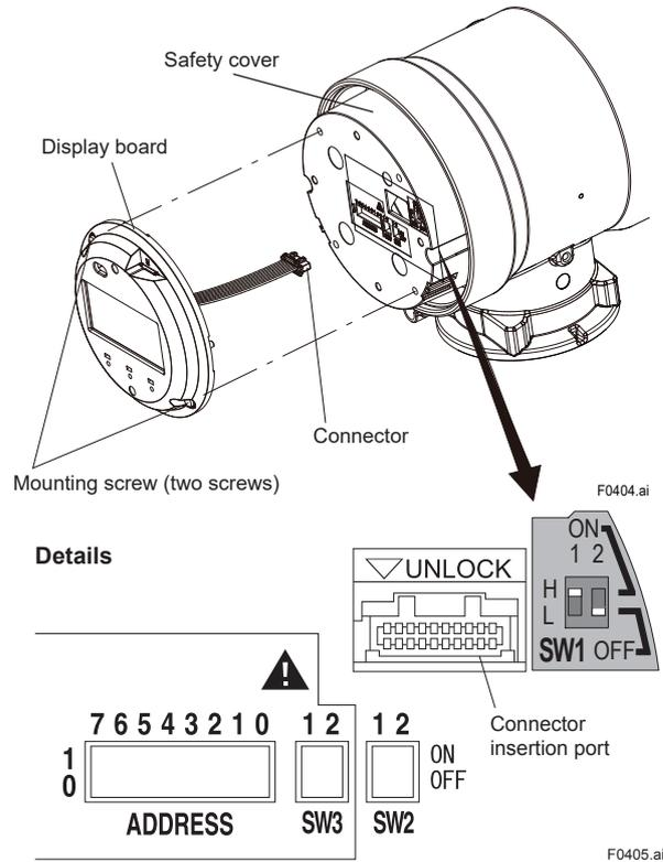
Figure 4.3 Connector Insertion Port of Display Board
