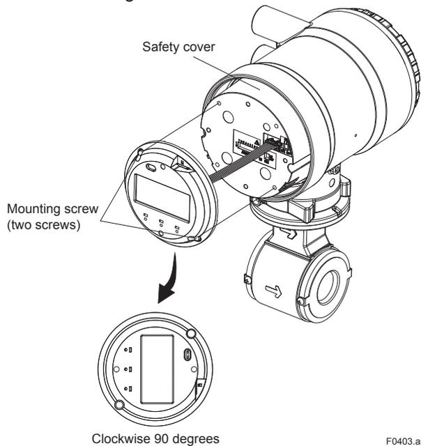
Figure 4.1.3 Changing Display Unit Direction 90 degrees
