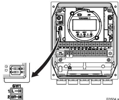
**Figure 5.4 Hardware switches (SW1-1, SW1-2)**
