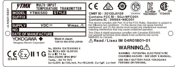
Figure 2.6 Name plate for IECx intrinsically safe explosion-proof transmitter (Battery Mode)
